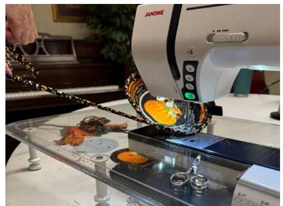
Attaching the coil to the fabric bottom is key step in making a rope bowl.
